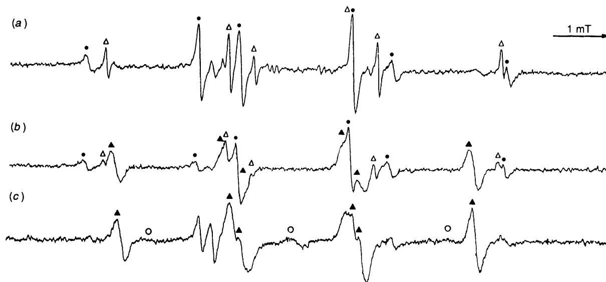
Fig. 1 EPR spectra of the radicals produced during the hydroxyl-initiated polymerization of acrylic acid at pH ca. 2, showing the variation in the concentration of \cdot\text{CH}_2\text{CH}(\text{OH})\text{CO}_2\text{H} ( \Delta ), \cdot\text{CH}(\text{CO}_2\text{H})\text{CH}_2\text{OH} ( \bullet ), dimer (and trimer) ( \blacktriangle ) and mid-chain ( \circ ) radicals with concentration of acrylic acid; [\text{Ti}^{\text{III}}] = 1.67 \times 10^{-3} \text{ mol dm}^{-3} , [\text{H}_2\text{O}_2] = 1.67 \times 10^{-2} \text{ mol dm}^{-3} ; [\text{AA}] = 4 \times 10^{-3} (a), 1.5 \times 10^{-2} (b), 4.8 \times 10^{-2} \text{ mol dm}^{-3} (c)
